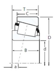
35 mm x 72 mm x 28,575 mm KBC TR357228HL tapered roller bearings
